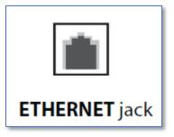
This is the simplest and most reliable way to connect your Smart TV to the internet. If your Smart TV has a wired connector, it will have a jack on the back of the TV that looks like this. If you're Smart TV doesn't have this connection, skip down to the *Wi-Fi Connection* instructions.
