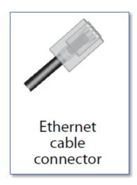
To connect it, you will need a network cable that looks like this on both ends. Note that it has *eight* wires and is not a regular telephone cable. Often these come with your internet router and just get left in the box. Sometimes they even come with Smart TVs.
